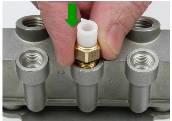
Fig. 13: Positioning the assy at right angles
