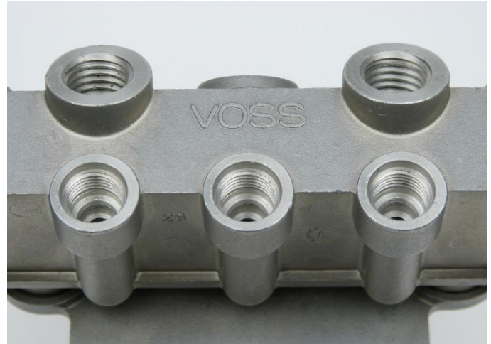
Fig. 14: Clean and correct connecting bores
