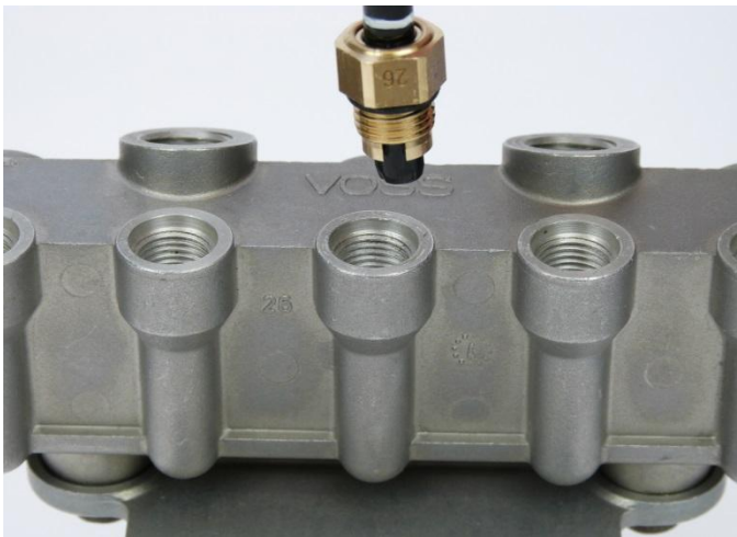
Fig. 28: Disconnected tube with assy
